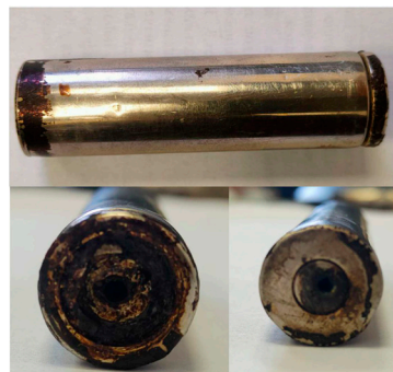
Fig. 1. Sample of the Panasonic NCR18650 lithium-ion battery with internal filling and holes for placing thermocouples
