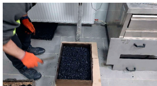
Fig. 5. The process of molding asphalt concrete beam specimens
