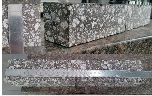
Fig. 6. Beam specimen for four-point bending tests
