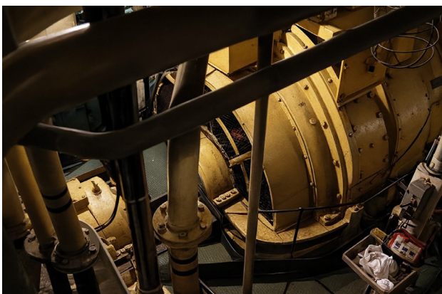
Fig. 5. Traction induction motor for the propeller drive of the vessel's propulsion power plant Caterpillar 3516
