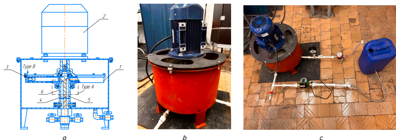
Fig. 1. Alternative inertial hydrodynamic installation: a – section of the installation; b – general view of the installation; c – test bench: 1 – rotor, 2 – electric motor, 3 – central fixed disk, 4, 5 – coolant supply and discharge channels, 6 – fixed rack
