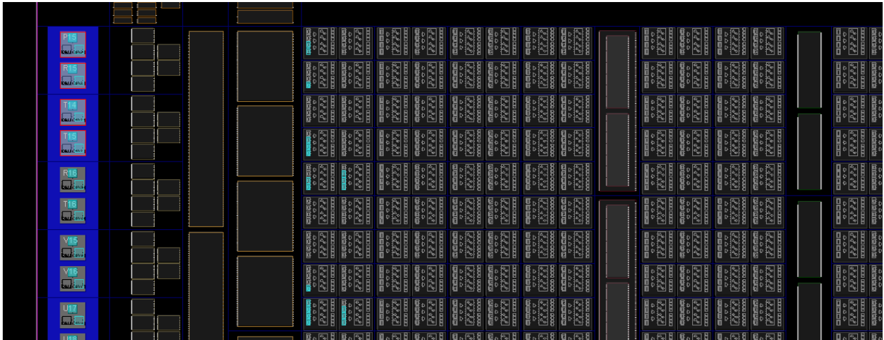
Fig. 17. Internal part of the xc7a50tcsq324-1 crystal when implementing a 64-bit cascade adder
