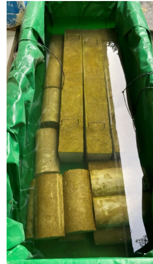
Fig. 4. Immersion process of cylindrical concrete specimens
