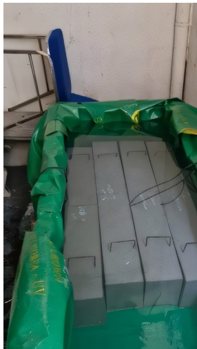
Fig. 2. Immersion process of concrete beams
