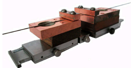
Fig. 4. Device for fixing and compressing elements during the welding process
