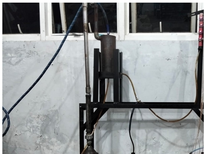
Fig. 1. Updraft gasifier: a – schematic experiment; b – experimental setup
