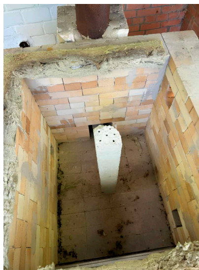
Fig. 2. Fragment of a reinforced concrete column made in a small-sized fire furnace
