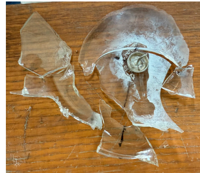
Fig. 5. Brittle fracture of the glass dome with crack initiation in the upper zone
