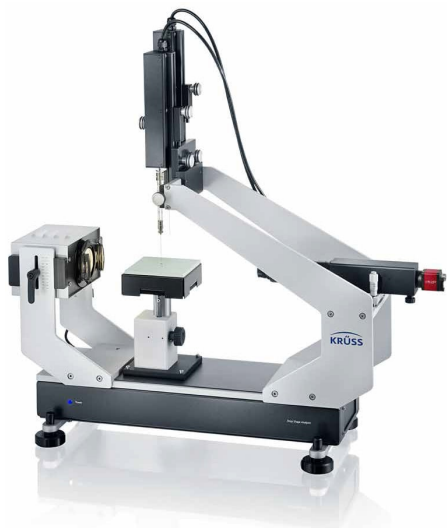
Fig. 1. General view of the contact angle measuring device DSA25, Krüss (Germany)
