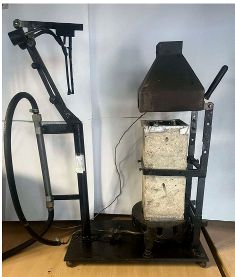
Fig. 1. Test furnace according to GOST 16363-98
