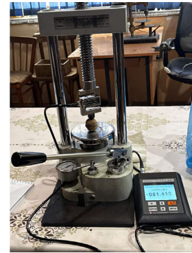
Fig. 5. Determining the maximum breaking force in Newtons of a walnut without a cleft using a special device
