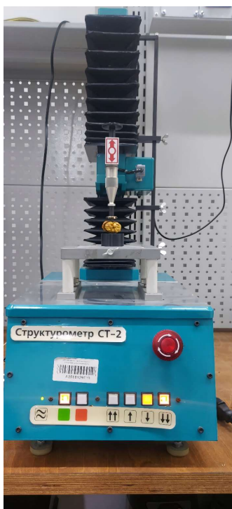
Fig. 8. Structure meter ST2 for determining the crushing force of walnut kernels
