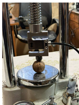
Fig. 4. Determining the maximum breaking force of a walnut with a cleft on a special device
