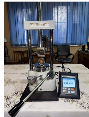
Fig. 6. A device for determining the breaking force between rough surfaces with a pitch of protruding elements of 10, 13, 16 mm from the side of a natural crack
