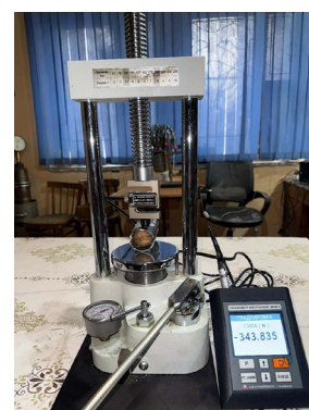
Fig. 7. Device for determining the breaking force between rough surfaces with a pitch of protruding elements of 10, 13, 16 mm from the side of a solid shell
