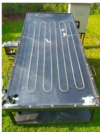
Fig. 4. Flat plate solar collector temperature measurement using type K thermocouples
