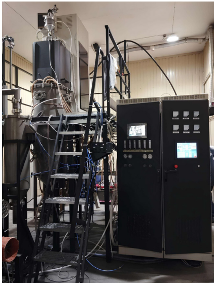
Fig. 1. Installation of inductively coupled plasma spheroidization of powders
