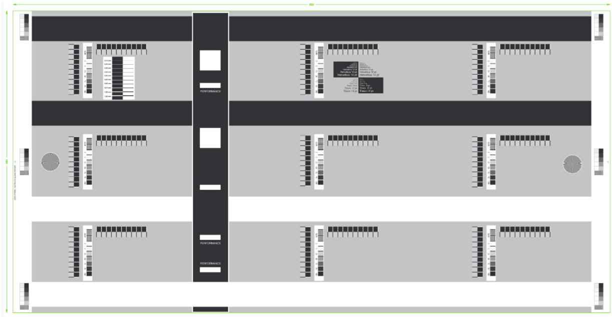
Fig. 2. Placement of test elements on the printing plate along the width of the print (left, center and right zones)
