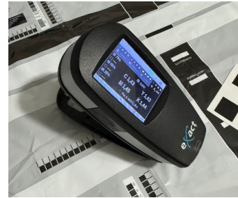
Fig. 1. Illustration of the optical density measurement process with an eXact spectrodensitometer
