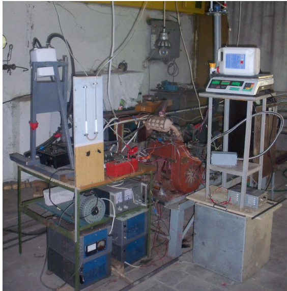
Fig. 1. General view of the experimental bench based on the spark-ignition engine 2Ch 7.2/6
