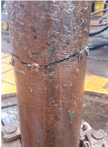
Fig. 2. The crack location of the fractured drill pipe
