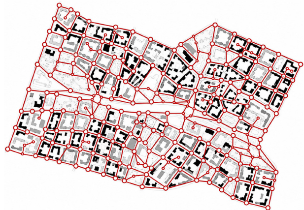
Fig. 1. Simulation model of the logistics environment of the construction site of a quarter-city development
