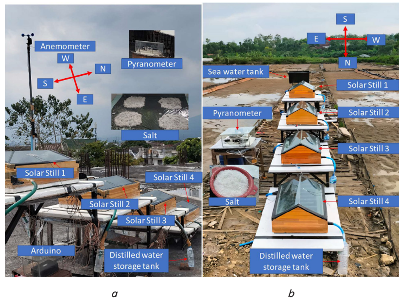
Fig. 1. Experimental setup of the multi-stage double-slope solar still at two testing sites: a – Solar and Alternative Energy Laboratory, Widya Gama University, Malang; b – Perseroan Terbatas Garam Dua Musim, Lamongan
