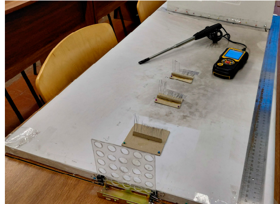
Fig. 4. Physical model of a perforated screen
