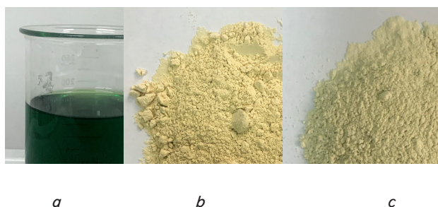
Fig. 1. \text{FePO}_4 preparation: a – electrolyte with dissolved metal; b – dried \text{FePO}_4 ; c – sintered \text{FePO}_4
