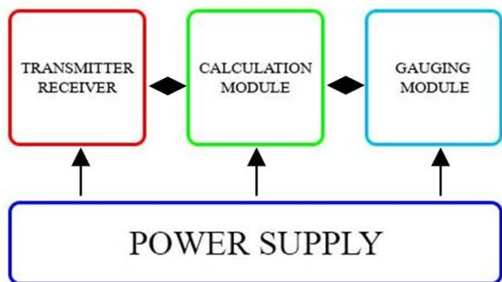
Fig. 3. A standard sensor node within a wireless network
