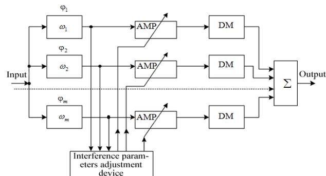
Fig. 2. Structural scheme of the adaptive receiver of the parallel complex signal:  $\varphi_1, \varphi_2, \dots, \varphi_m$  – voice filters;  $\omega_1, \omega_2, \dots, \omega_m$  – voice filters frequencies; AMP – amplifiers; DM – demodulators;  $\Sigma$  – adder
