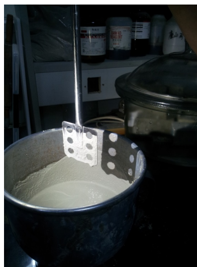
Fig. 1. Determination of flowability (VISUAL ASSESSMENT) with a special testing equipment (a paddle with openings)
