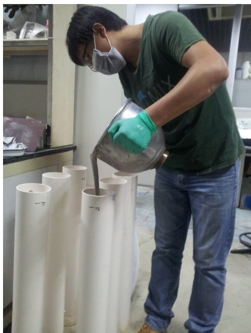
Fig. 2. Filling moulds with the grout (cylinder specimens: d=120 mm and h=800 mm)
