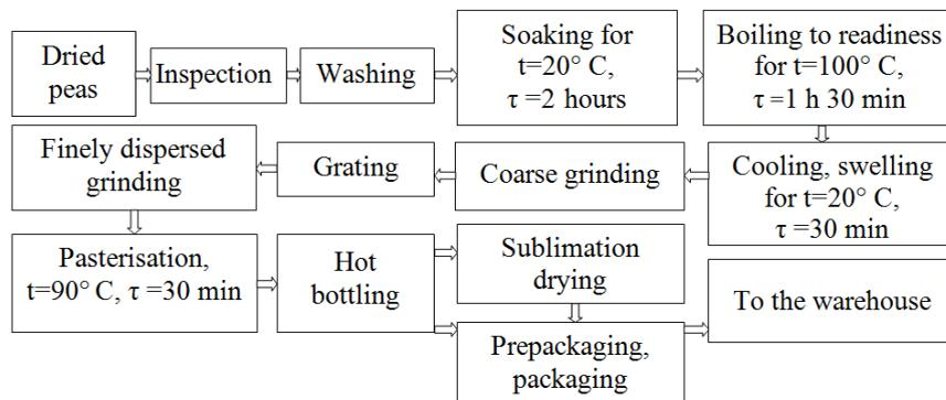
Fig. 3. Technological scheme of obtaining nanostructured puree and nanopowders with prebiotic properties of peas, using steam and thermal processing and non-enzymatic biocatalysis
