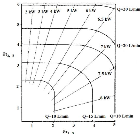
Fig. 7. Nomogram for determining parameters of pulse  $\delta\tau_1$  and  $\delta\tau_2$  depending on the flushing fluid consumption Q and down-hole power
