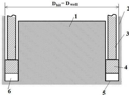
Fig. 2. 3D model of the estimated area: 1 – core; 2 – wall of a well; 3 – drilling bit body; 4 – matrix; 5 – surface of a working face; 6 – flushing channel
