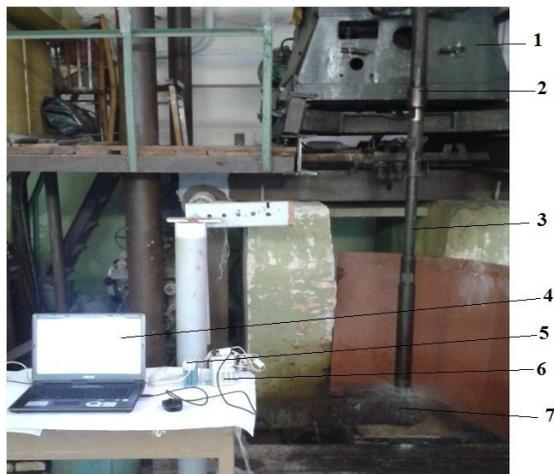
Fig. 3. General view of experimental bench: 1 – drilling machine ZIF–650M; 2 – lead pipe; 3 – drilling tools; 4 – laptop PC; 5 – charger for modules WAD-AIK-BUS (USB); 6 – analog-digital converter WAD-AIK-BUS (USB); 7 – granite block
