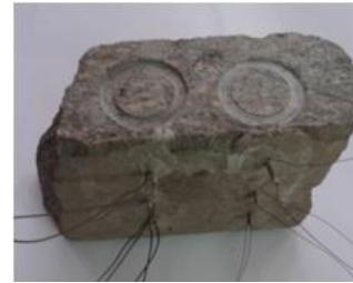
Fig. 4. Block of rock with thermocouples
