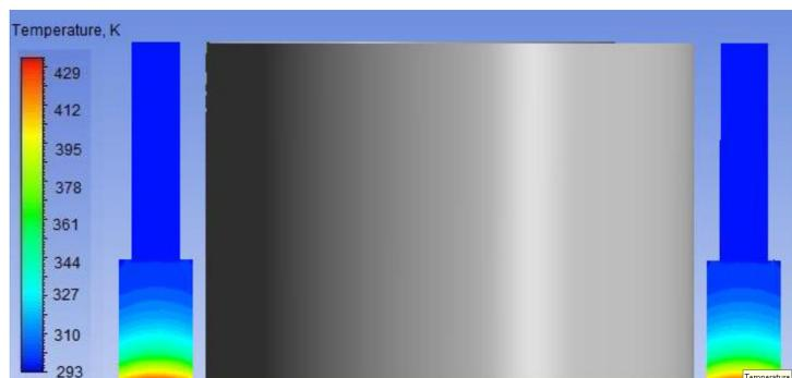
Fig. 6. The results of calculation of temperature field on the working face during drilling
