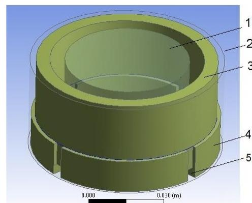
Fig. 1. General view of a diamond drilling bit: 1 – core; 2 – wall of a well; 3 – drilling bit body; 4 – matrix; 5 – flushing channel
