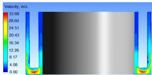
Fig. 5. The results of calculation of velocity field on the working face during drilling
