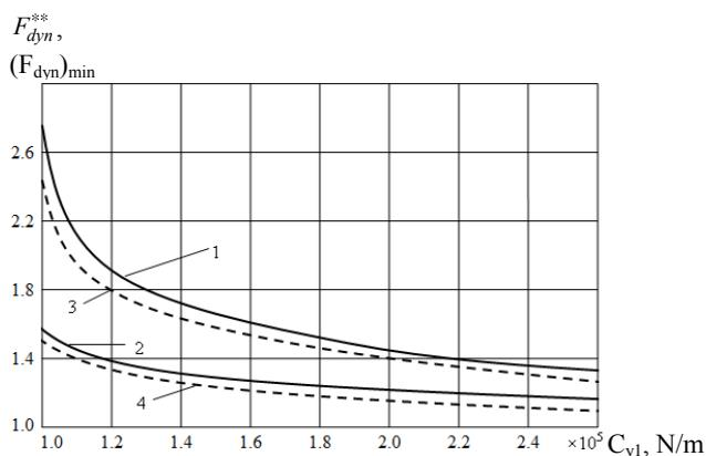
Fig. 3. The dependence of the dynamic factor on the total lateral rigidity of the front wheel tires: 1 and 2 –  $F_{dyn}^{**}(C_{y1})$ ; 3 and 4 –  $(F_{dyn})_{min}(C_{y1})$ ; 1 and 3 – a loaded vehicle Ural-4320; 2 and 4 – an equipped vehicle Ural-4320
