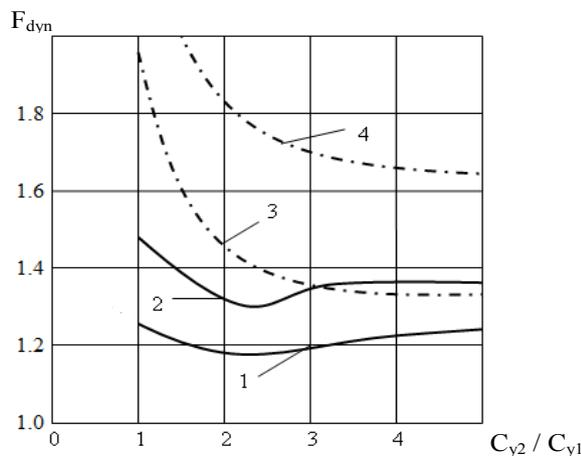
Fig. 2. The dependence of the dynamic factor on the relationship  $C_{y2}/C_{y1}$ ; 1 and 2 denote an equipped vehicle; 3 and 4 denote a fully loaded vehicle; 1 and 3 refer to  $C_{y1}=2.264 \cdot 10^5$  N/m; 2 and 4 refer to  $C_{y1}=1.475 \cdot 10^5$  N/m
