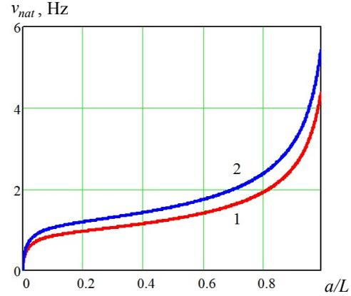
Fig. 1. The dependence  $v_{nat} \left( \frac{a}{L} \right)$  for vehicles with a neutral steering:  $m_a=8,100$  kg;  $L=4.2$  m;  $B=2.0$  m;  $C_{y1}=1.475 \times 10^5$  N/m (curve 1) and  $C_{y2}=2.264 \times 10^5$  N/m (curve 2)
