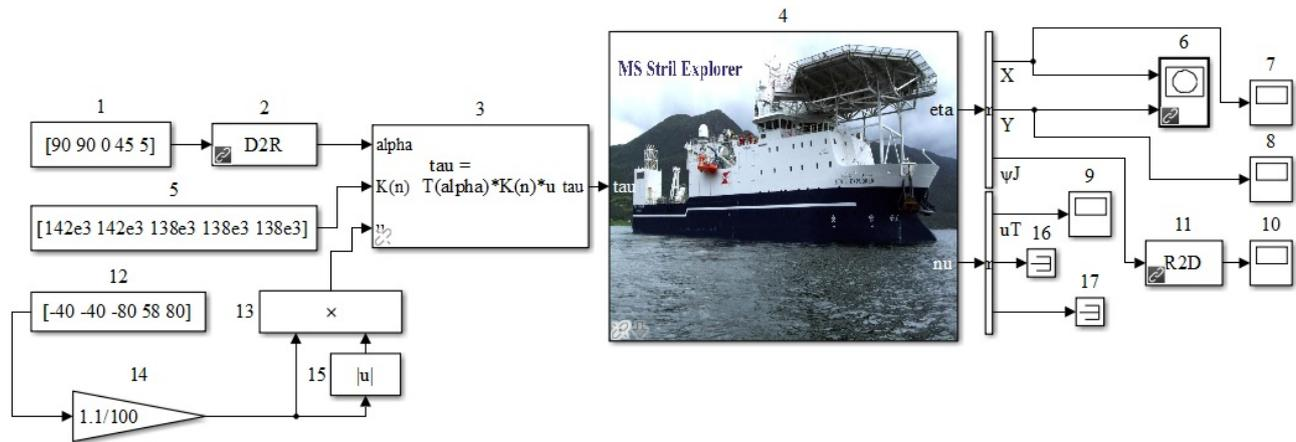
Fig. 3. Computer simulation in MatLab Simulink of the configuration of thrusters for the ship of the type Supply Vessel:
