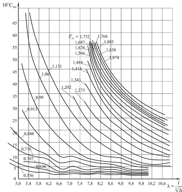
Fig. 1. Experimental dependencies of the ratio of resistance on a ton of water tonnage in the function of coefficient of longitudinal hull sharpness and Froude's number
