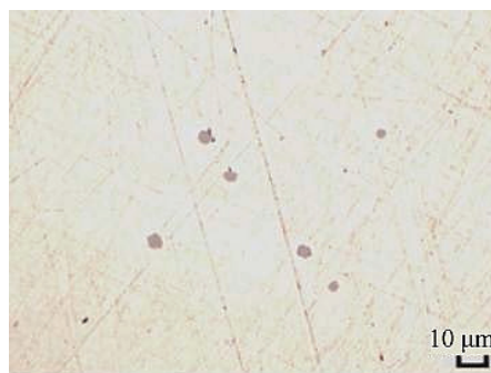
Fig. 4. Lamellar (a) and spherical (b) IC in ML5 alloy
