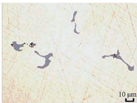
Fig. 4. Lamellar (a) and spherical (b) IC in ML5 alloy
