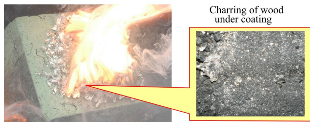
Fig. 5. The results of testing the model sample treated with organic-mineral compounds based protective coating
