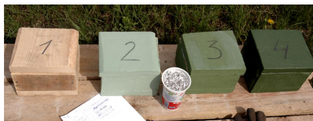
Fig. 1. Model patterns of wooden structures: 1 – untreated one, 2 – fire retardant coating on organic-mineral bases; 3 – fire retardant coatings based on inorganic compounds [9]; 4 – geocement refractory fire retardant coatings with heat reflecting screens
