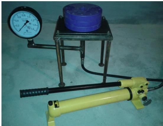
Fig. 3. A calibration unit: *a* – the schematic diagram of the unit: 1 – a load, 2 – a rubber sample, 3 – a base plate, 4 – a changeable insert and 5 – a test hole; *b* – the general view of the calibration unit
