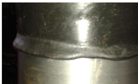
Fig. 9. The results of squeezing the ring support section into a 3 mm clearance after the post-experimental withdrawal of the packer from the laboratory model
