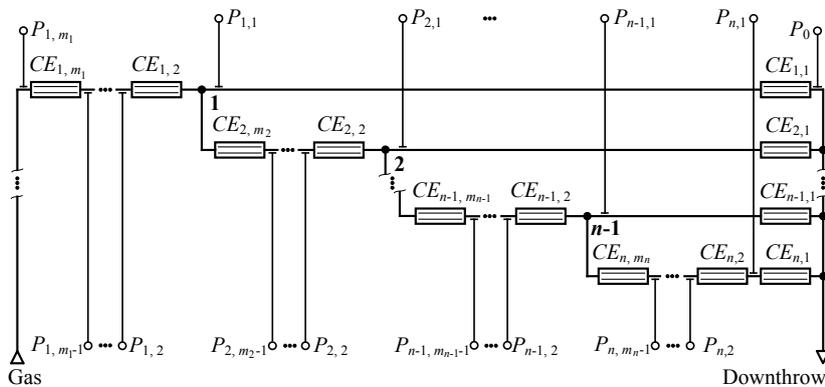
Fig. 4. Generalized principal scheme with binary ramification of dividers for setting low pressures (drops)
