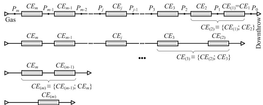
Fig. 2. Multi-capillary pressure divider and  $m-1$  of its equivalent transformations
