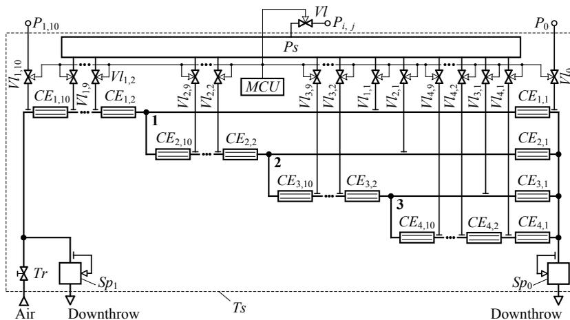
Fig. 5. Schematic of a four-decade pressure setting device:  $Ps$  is the pneumatic switch;  $MCU$  is the microprocessor control unit;  $Vl_{i,j}$  is the electromagnetic valve, set up on the line of pressure selection  $P_{i,j}$  from the inter-throttle chamber, formed by capillaries  $CE_{i,j+1}$  and  $CE_{i,j}$ ;  $Tr$  is the alternative throttle;  $Ts$  is the thermostat;  $Sp_1$ ,  $Sp_0$  are the stabilizers of absolute pressure
