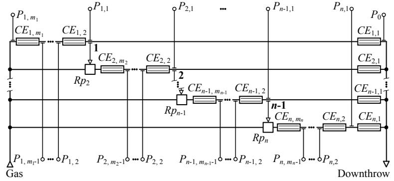
Fig. 3. Generalized schematic diagram of cascade connection of pressure dividers to set the pressures, different in magnitude (drops)
