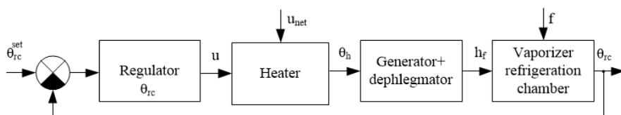
Fig. 1. Structural scheme of standard SAC of ARD
