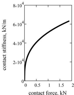
Fig. 8. Parametric characteristic of contact rigidity and strength in the intermediate supports during displacement of the local mass
