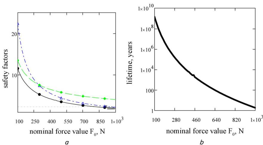
Fig. 9. Effect of nominal value of the effort: a – on the strength margin factors, ● –  $n$ , ◆ –  $n_c$ , △ –  $n_g$ ; b – on the spring’s lifetime
