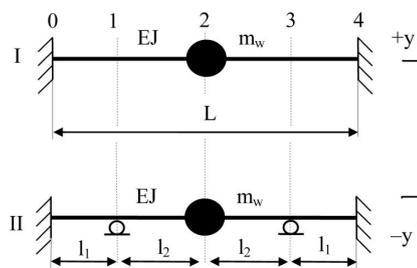
Fig. 1. Schematic of realization of asymmetric piecewise linear elastic characteristic on one flat spring
