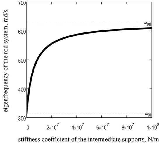
Fig. 4. Influence of coefficient of rigidity of the intermediate supports on the own oscillations frequency of the rod system
