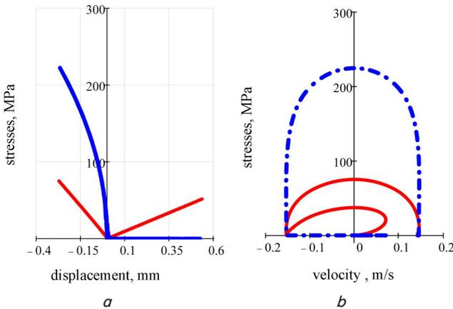
Fig. 7. Parametrical dependency of stress on kinematic parameters of the local mass: *a* – displacement; *b* – acceleration: red color – bending stress, dark blue color – contact stress
