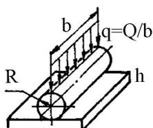
Fig. 2. Schematic of the contact problem
