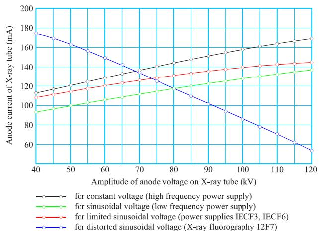
Fig. 5. Dependences of integral anode current of X-ray tube on the amplitude of applied voltage
