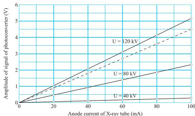
Fig. 2. Dependence of amplitude of the output signal of photo recorder on the anode current at different values of voltage on X-ray tube
