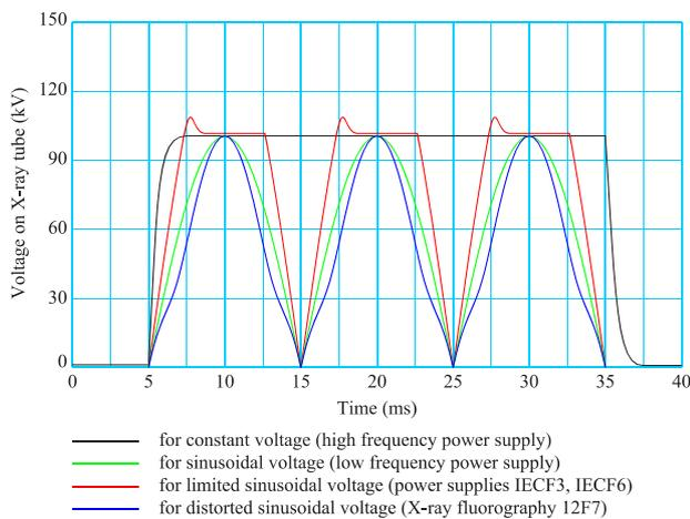
Fig. 4. Form of voltage on the X-ray tube when using different types of power sources
