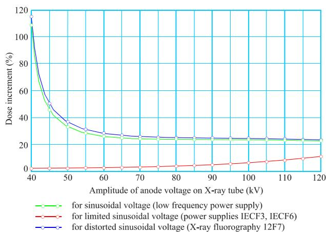
Fig. 9. Dependences of the equivalent dose increment on the amplitude of applied voltage relative to the dose, obtained when powered by direct current, for different power supply sources under condition of achieving the same level of X-ray image processing
