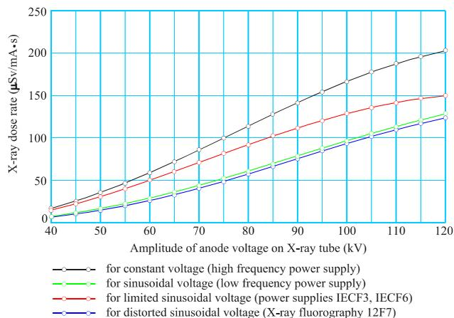
Fig. 6. Dependences of equivalent dose rate on the amplitude of applied voltage for the anode current 1 mA
