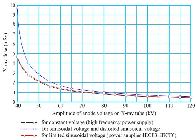
Fig. 8. Dependences of equivalent dose on the amplitude of applied voltage for various power sources, provided the same mean integral level of the blackening of film
