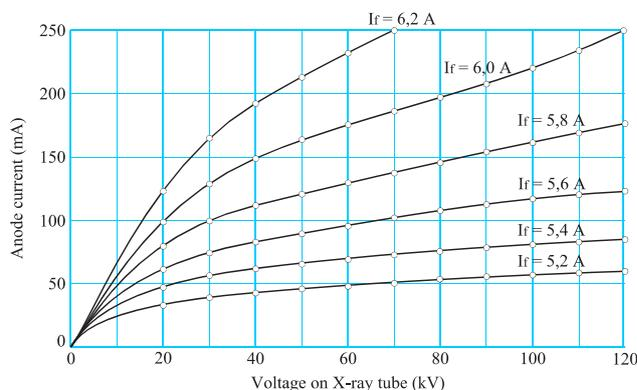
Fig. 1. Family of volt-ampere characteristics of X-ray tube
