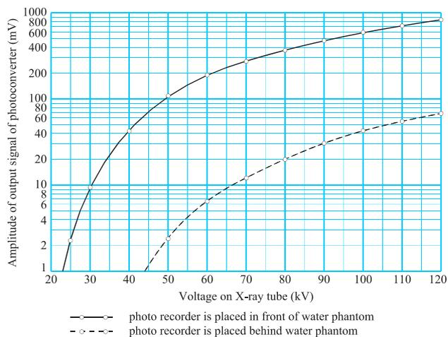
Fig. 3. Dependence of amplitude of output signal of photo recorder on the voltage on X-ray tube at its various positions
