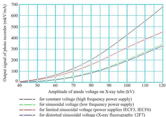
Fig. 7. Dependences of value of the mean integral brightness of the glow of the converting screen on the amplitude of applied voltage
