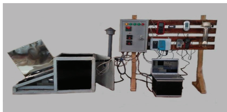
Fig. 1. Solar dryer with thermal battery and flat mirror concentrator: a – design and technological scheme; b – general view; 1 – input channel; 2 – fan with heater; 3 – air duct; 4 – air collector; 5 – heat accumulating material (pebble); 6 – drying chamber; 7 – return channel; 8 – sieves; 9 – flat mirror concentrator; 10 – valve
