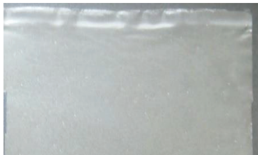
Fig. 2. Sample of film made of starch, gelatin and one of studied plasticizers
