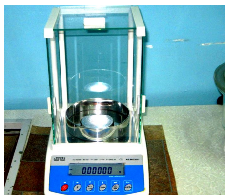
Fig. 1. General view of the analytical scales AS Radwag-60/220/S
