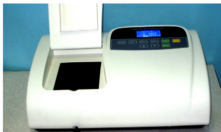
Fig. 3. General view of the spectrophotometer ULAB 102
