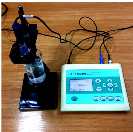
Fig. 2. General view of the ionomer I-160MI
