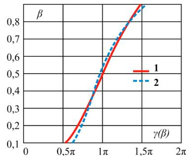
Fig. 5. Relationship between the coefficient of filling the drum and central angle of the segment with product: 1 – equation (9); 2 – approximate equation (26)
