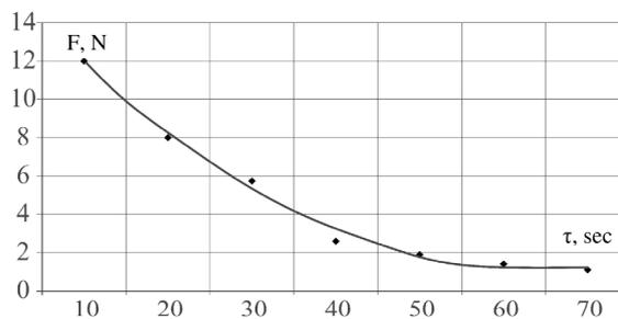
Fig. 7. Dependence of the effort of removing the husk of onion on the duration of its steam treatment
