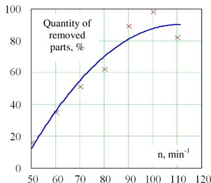
Fig. 12. Determining optimal drum rotation frequency by the indicator of quantity of removed parts of a bulb: × – experimental research; — – correlation curve
