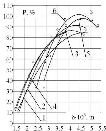
Fig. 9. Influence of the thickness of penetration through the surface layer of bulb on the degree of cleaning the bulbs at load factor 0.3 and shape and diameter of openings: 1 – circle, 12 mm; 2 – circle, 17 mm; 3 – circle, 22 mm; 4 – ellipse, 12×18 mm; 5 – ellipse, 17×23 mm; 6 – ellipse, 22×28 mm
