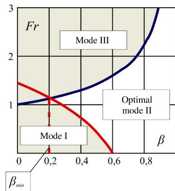
Fig. 6. Dependence of the Froude number's limiting values on the coefficient of filling the drum with onion
