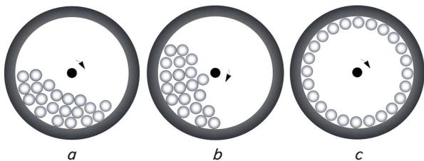
Fig. 2. Scheme of motion of solid particles in the drum depending on the rotation frequency: *a* – mode I,  $n=0,4...0,6 n_{cr}$ ; *b* – mode II,  $n=0,6...0,8 n_{cr}$ ; *c* – mode III,  $n \geq n_{cr}$
