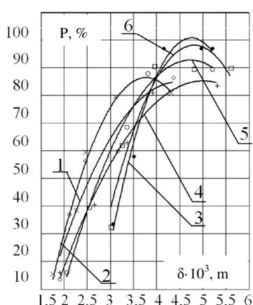
Fig. 10. Influence of the thickness of penetration through the surface layer of bulb on the degree of cleaning the bulbs at load factor 0.5 and shape and diameter of openings: 1 – circle, 12 mm; 2 – circle, 17 mm; 3 – circle, 22 mm; 4 – ellipse, 12×18 mm; 5 – ellipse, 17×23 mm; 6 – ellipse, 22×28 mm
