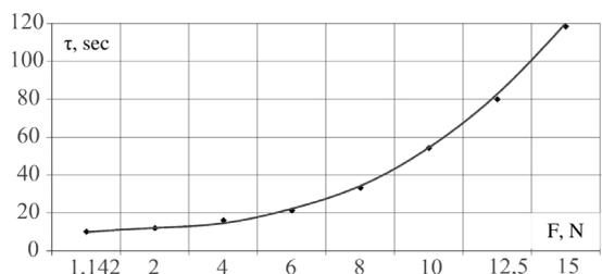
Fig. 8. Dependence of duration of mechanical cleaning of napiform onion on the effort to remove its husk
