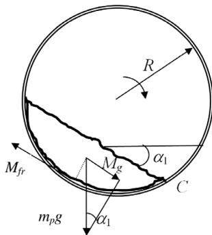
Fig. 4. Scheme of the forces that determine angle of lifting the layer of product  $\alpha_1$  under the first mode of the drum operation
