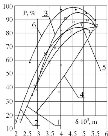
Fig. 11. Influence of the thickness of penetration through the surface layer of bulb on the degree of cleaning the bulbs at load factor 0.7 and shape and diameter of openings: 1 – circle, 12 mm; 2 – circle, 17 mm; 3 – circle, 22 mm; 4 – ellipse, 12×18 mm; 5 – ellipse, 17×23 mm; 6 – ellipse, 22×28 mm
