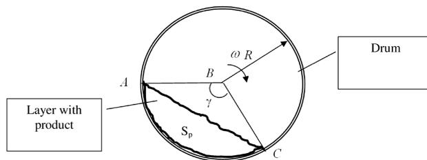
Fig. 3. Scheme of position of the layer of onion in the drum
