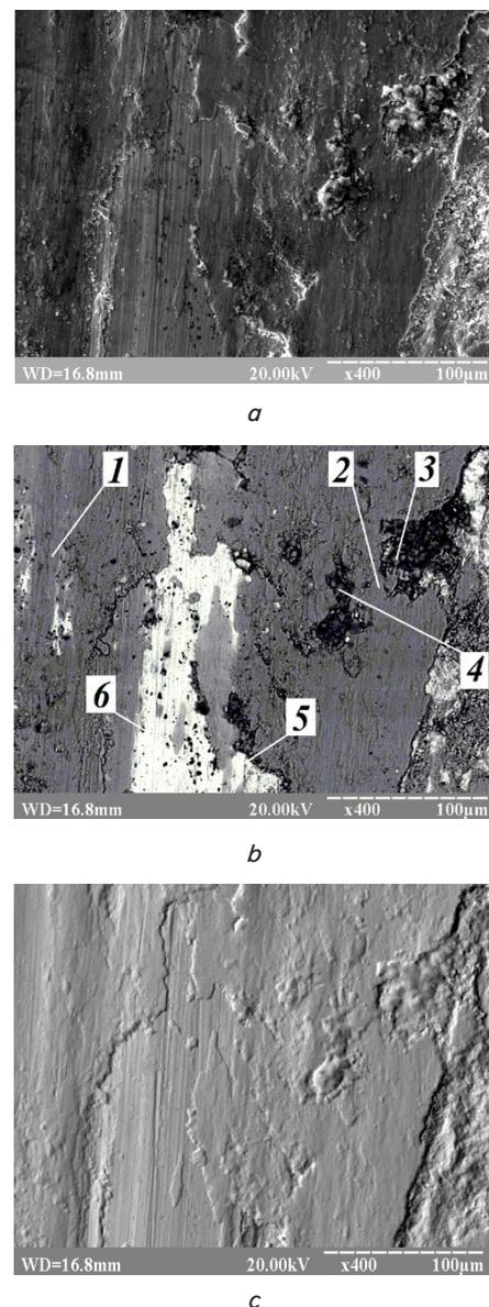
Fig. 5. Microstructure  $\times 400$  of the section of friction surface of coating at 250 °C: *a* – in reflected; *b* – in secondary; *c* – surface topography with the indication of sections of micro X-ray spectral analysis at. % in Table 2
