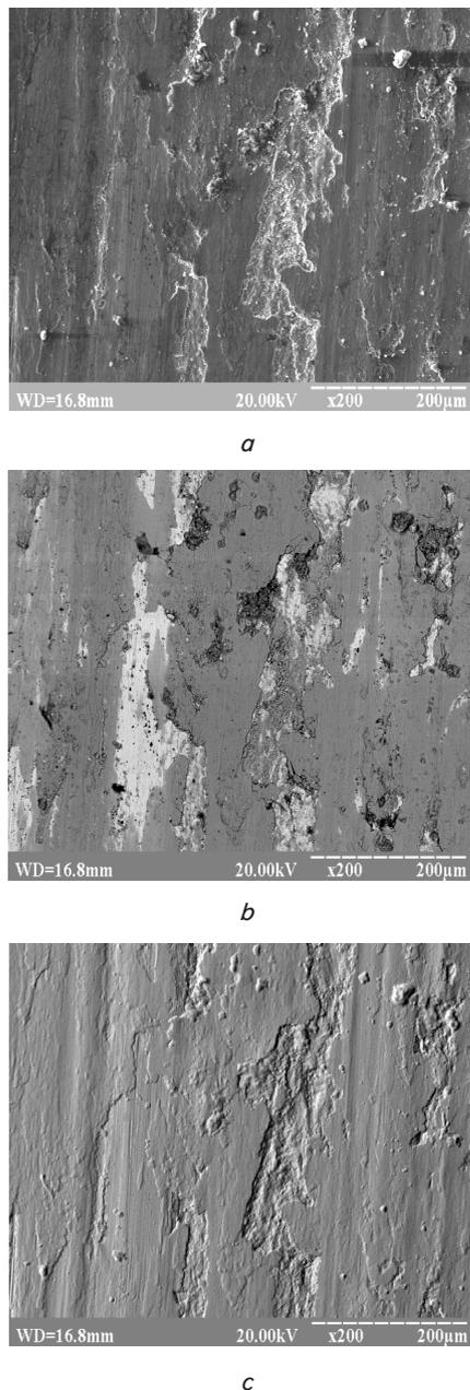
Fig. 4. Friction surfaces of coating of the (SiC–Al<sub>2</sub>O<sub>3</sub>)-FeSi system at magnification 200 with a temperature of 250 °C: *a* – in reflected electrons; *b* – in secondary electrons; *c* – surface topography
