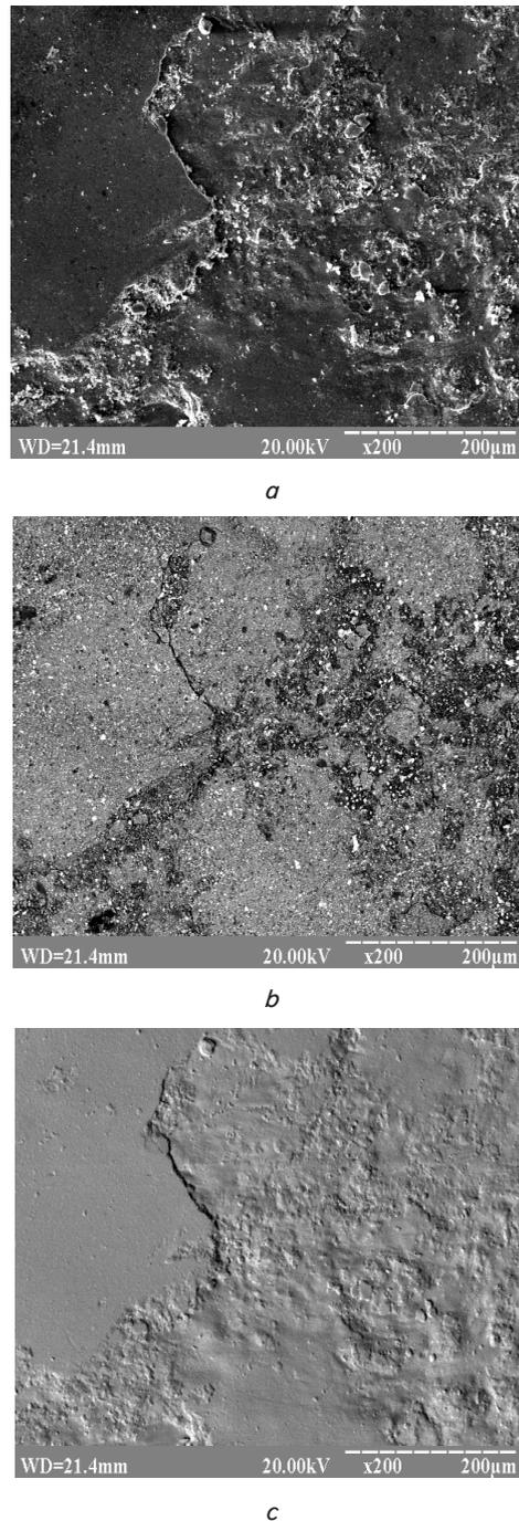
Fig. 6. Friction surfaces of coating of the  $(\text{SiC}-\text{Al}_2\text{O}_3)-\text{FeSi}$  system at magnification 200 at temperature 500 °C: *a* – in reflected electrons; *b* – in secondary electrons; *c* – surface topography
