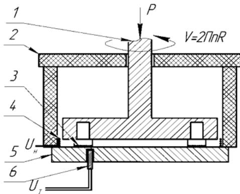
Fig. 1. Schematic of friction node of plant with heating: 1 – shaft of machine; 2 – heatproof housing; 3 – sample with coating; 4 – heating element; 5 – counterbody; 6 – thermocouple
