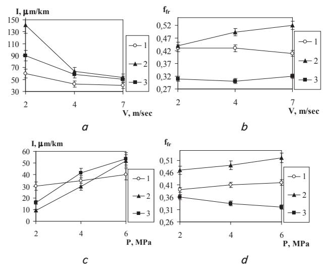
Fig. 3. Dependence of wear intensity and friction coefficient of plasma coating of the (SiC–Al<sub>2</sub>O<sub>3</sub>)–FeSi system: *a*, *b* – on speed; *c*, *d* – on load; at different temperatures: 1 – without heating; 2 – 250 °C; 3 – 500 °C
