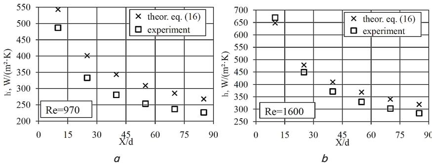
Fig. 3. Dependence of local heat-transfer coefficient lengthwise initial thermal section at the forced motion of distilled water in the pipe at  $d=0.01$  and  $l=0.85$  m:  $a - Re=970$ ;  $b - Re=1600$
