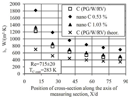
Fig. 5. Dependence of local heat-transfer coefficient lengthwise the initial thermal section at the forced motion of coolants in the pipe ( $d=0.01$  and  $l=0.85$  m)
