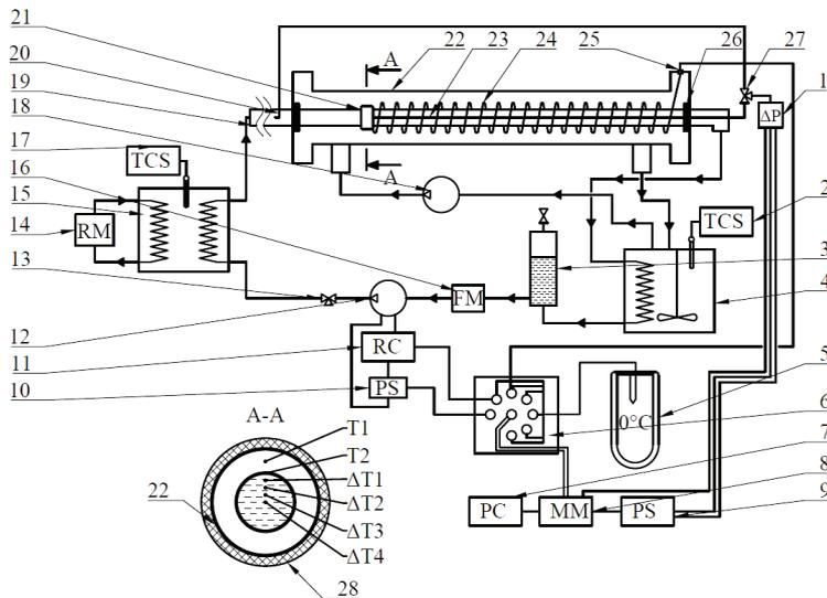
Fig. 1. Schematic diagram of experimental installation “pipe in a pipe”
