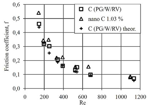
Fig. 7. Dependence of friction coefficient lengthwise on the Reynolds number for the base coolant (PG/W/R) and nanofluid of the nanoC 1.03 %
