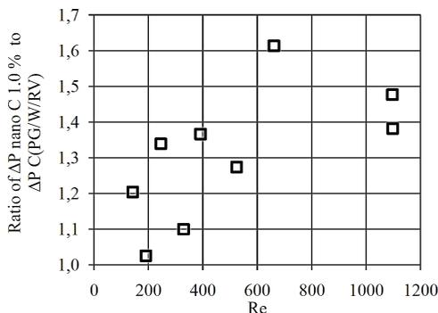
Fig. 6. Dependence of ratio of pressure losses for the nanoC 1.0 % to pressure losses for the base coolant C (PG/W/RV) on the Reynolds number
