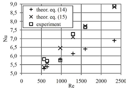
Fig. 2. Dependence of the mean value of Nusselt number on the Reynolds number at the forced motion of distilled water in the pipe at  $d=0.01$  and  $l=0.85$  m (initial thermal section)
