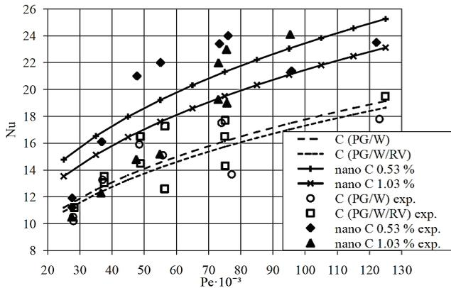
Fig. 4. Dependence of the mean Nusselt number values on the Peclet number at the forced motion of coolants in the pipe at  $d=0.01$  and  $l=0.85$  m (initial thermal section) for the coolant PG/W, base coolant PG/W/RV and nanofluids of the nanoC 0.53 % and the nanoC 1.03 %
