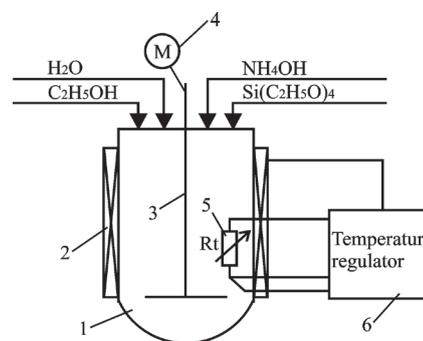
Fig. 1. Manufacturing section for the synthesis of  $\text{SiO}_2$  particles by the hydrolysis of TEOS with different storage period: 1 – reactor; 2 – heating element; 3 – mixer; 4 – electric motor; 5 – thermistor; 6 – regulator
