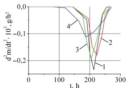
Fig. 6. Increase in the sediment mass in the sedimentation process of  $\text{SiO}_2$  particles synthesized from TEOS with different storage periods: 1 – immediately after fractional distillation; 2 – in 48 hours after TEOS purification; 3 – in 96 hours after TEOS purification; 4 – in 144 hours after TEOS purification
