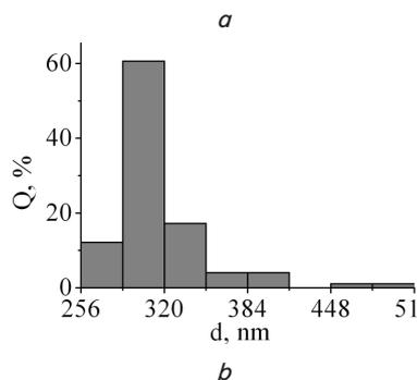
Fig. 3. Histogram of diameter distribution of synthesized particles *d* depending on the relative amount of particles in the interval of column of in histogram *Q*: *a* – particles, suitable for the formation of photonic crystal; *b* – particles that do not form photonic crystal
