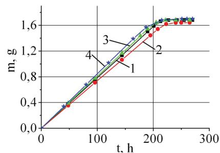
Fig. 5. Sedimentation curves of suspensions (dependence of sediment mass  $m$  on the settling time  $t$ ) synthesized from tetraethoxysilane with different storage periods: 1 – immediately after fractional distillation; 2 – in 48 hours after TEOS purification; 3 – in 96 hours after TEOS purification; 4 – in 144 hours after TEOS purification
