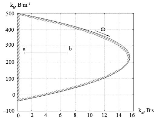
Fig. 2. Stability region and region of maximum stability margin of the closed fuel feed system
