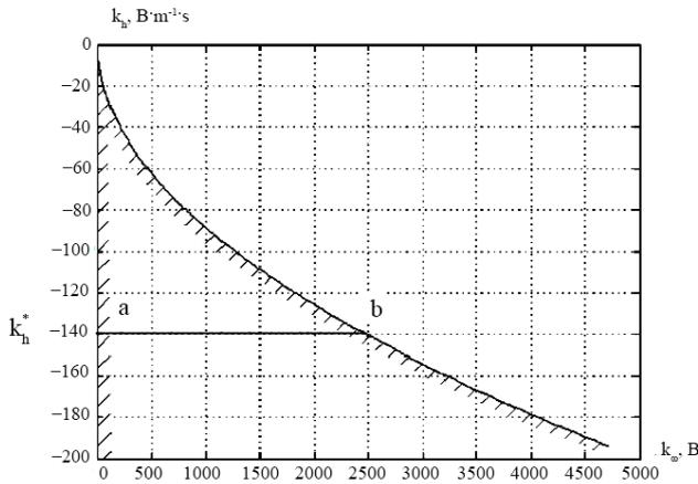
Fig. 4. Stability region of the closed fuel feed system
