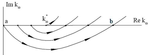
Fig. 5. Lines of equal stability level in the plane of comprehensive parameter  $k_\omega$
