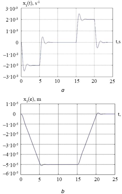
Fig. 7. Processes of working out external disturbances: *a* – process of changing angular velocity of crankshaft; *b* – process of changing a position of lath of fuel pump
