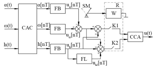
Fig. 8. Digital electronic control unit
