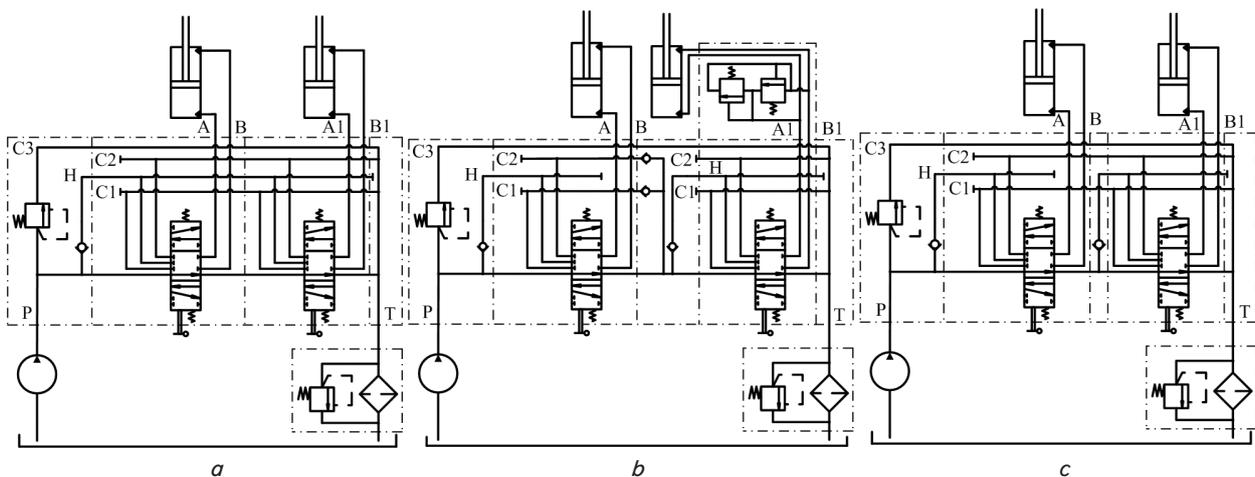
Fig. 4. Schemes of energy distribution from the pump to the hydraulic engines: a – parallel; b – sequential; c – individual. Designations in formulas (4) and (5) characterize the following: A, B, A1, B1 – cavities of hydraulic engines, the first and the second, respectively; C1, C2 – drain pipelines that are connected with the allocator; C3 – drain pipeline that is connected to the safety valve; H – pressure channel; P – total pressure provided by the pump; T – pressure in the drain pipeline
