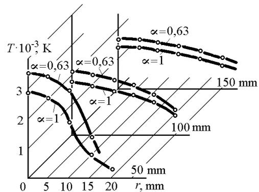
Fig. 7. Radial temperature distributions of plasma gas-air jet under condition of change in the composition of plasma-forming mixture ( $Q_{\Sigma}=3.5 \text{ m}^3/\text{h}$ )
