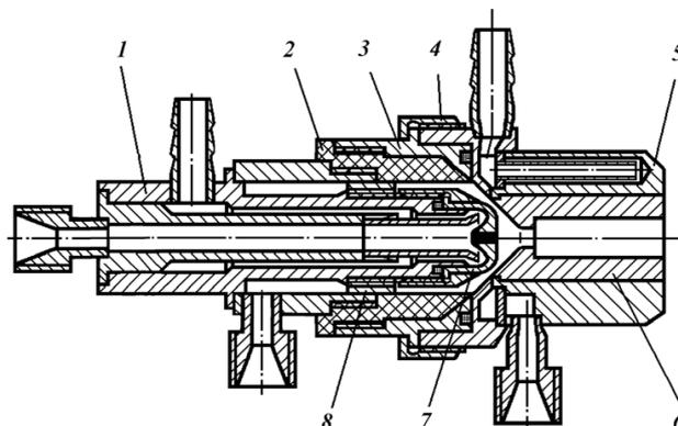
Fig. 1. Experimental plasma spray with a combined energy supply: 1 – cathode node; 2 – insulator; 3 – cup; 4 – union nut; 5 – anode node of middling cooling; 6 – output electrode-nozzle; 7 – thermal-chemical electrode (cathode); 8 – swirler
