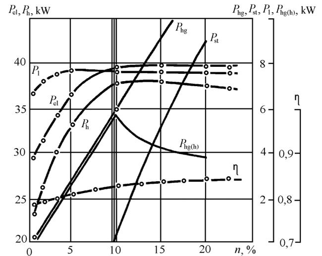
Fig. 3. Dependence of the components of capacity of plasma jet on the content of hydrocarbon component (methane) in the original plasma-forming mixture
