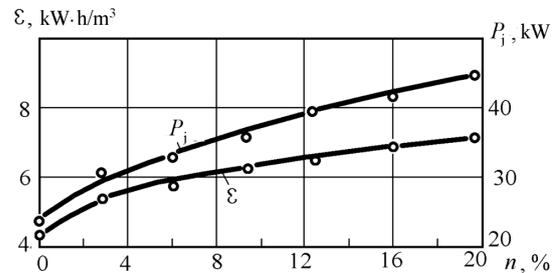
Fig. 9. Dependences of the total useful capacity and specific power of plasma jet on the content of hydrocarbon component in the original plasma-forming mixture (*I*=200 A, *Q*<sub>2</sub>=5.3 m<sup>3</sup>/h)
