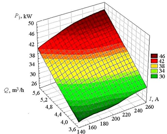
Fig. 5. Dependence of plasma jet capacity on the operational parameters of the gas-air plasma generation process ( $\alpha=0.4$ )
