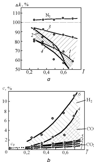
Fig. 2. Change in the content of components of the plasma-forming mixture along the arc channel of sprayer:  $a$  – starting methane content (CH<sub>4</sub>) 12 % (by volume): 1 – methane (arc current  $I=170$  A); 2 – CH<sub>4</sub> ( $I=250$  A); 3 – content of oxygen O<sub>2</sub> ( $I=170$  A); 4 – O<sub>2</sub> ( $I=250$  A);  $b$  – starting content of methane (CH<sub>4</sub>) 12 %: 1, 3, 5 –  $I=170$  A; 2, 4, 6 –  $I=250$  A
