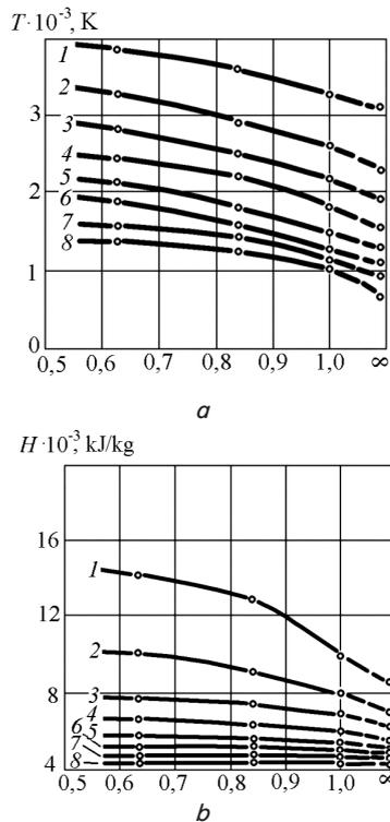
Fig. 8. Dependence of temperature and enthalpy on the coefficient of oxidizer consumption of plasma-forming mixture (along the longitudinal axis of plasma jet): *a* – dependence of temperature; *b* – dependence of enthalpy; 1 – distance of 40 mm; 2 – 60 mm; 3 – 80 mm; 4 – 100 mm; 5 – 120 mm; 6 – 140 mm; 7 – 160 mm; 8 – 180 mm (*I*=200 A; *Q*=6.3 m<sup>3</sup>/h; *P*=24 kW)
