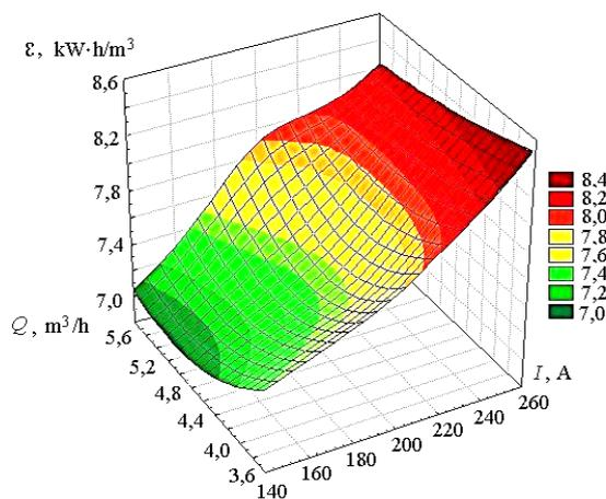
Fig. 4. Dependence of specific energy of plasma jet on the operational parameters of the gas-air plasma generation process ( $\alpha=0.4$ )
