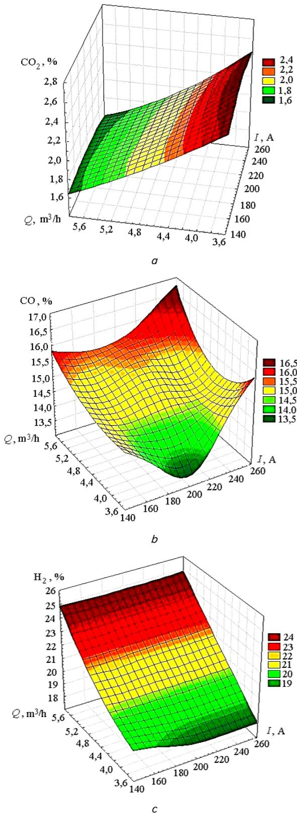
Fig. 6. Dependences of the content of basic components of gas jet on the operational parameters of plasma generation ( $\alpha=0.4$ ): a – carbon dioxide; b – carbon oxide; c – hydrogen
