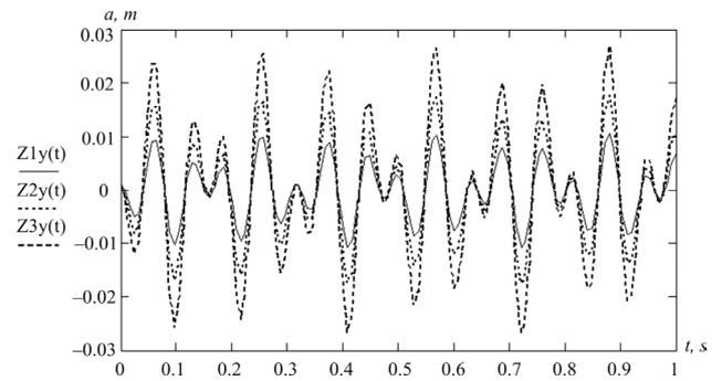
Fig. 3. Impact of the debalances radii on the magnitude of oscillation amplitude of the separator drum at  $Z1 - r_1 = r_2 = 0,045$  m,  $Z2 - r_1 = r_2 = 0,09$  m,  $Z3 - r_1 = r_2 = 0,135$  m
