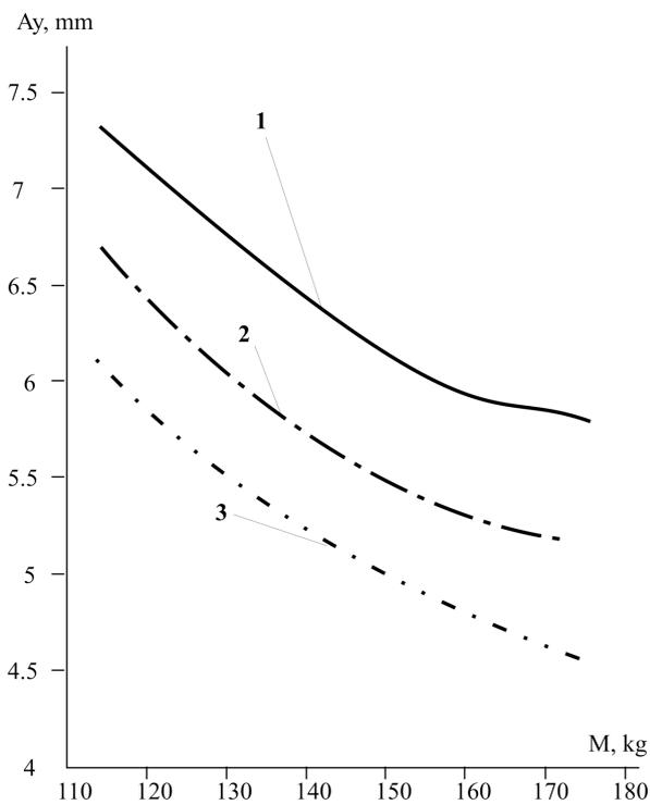
Fig. 7. Dependence of oscillation amplitude of vibratory separator on the oscillatory mass at the debalances angular velocity  $\omega_1=\omega_2=110 \text{ s}^{-1}$ : 1 – suspension rigidity 10 kN/m; 2 – 13 kN/m; 3 – 16 kN/m
