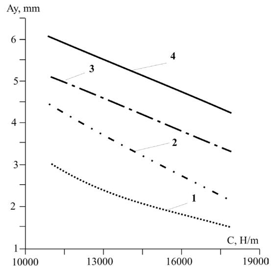
Fig. 8. Dependence of oscillation amplitude of vibratory separator on the magnitude of rigidity of the suspension springs: 1 – magnitude of the debalance radius (eccentricity) 0.015 m; 2 – 0.03 m; 3 – 0.045 m; 4 – 0.06 m
