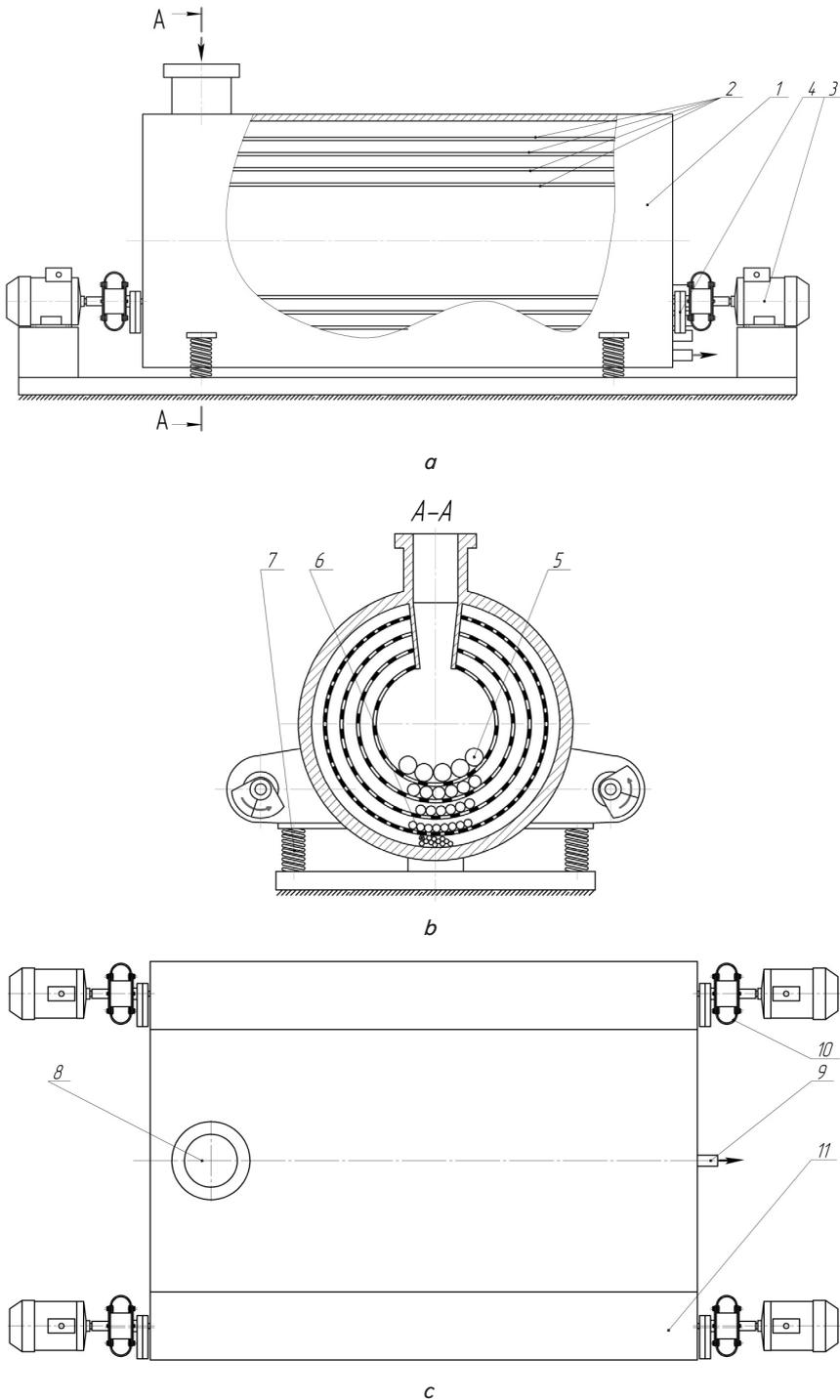
Fig. 1. Vibratory separator of the drum type with concentric arrangement of sieves and four debalances that have an independent drive: *a* – vibratory separator – main view; *b* – vibratory separator – side view (cross-section); *c* – vibratory separator – top view
