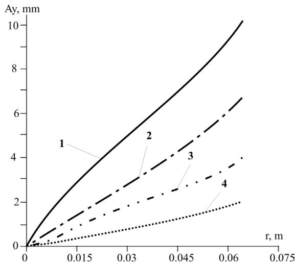
Fig. 6. Dependence of oscillation amplitude of vibratory separator on the radius of debalances: 1 – mass of debalances 8 kg; 2 – 6 kg; 3 – 4 kg, 4 – 2 kg
