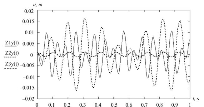
Fig. 5. Impact of the debalances rotation angular velocities on the magnitude of oscillation amplitude of the separator drum at  $Z1 - \omega_1 = 95$  s<sup>-1</sup>,  $\omega_2 = -95$  s<sup>-1</sup>,  $Z2 - \omega_1 = 50$  s<sup>-1</sup>,  $\omega_2 = -50$  s<sup>-1</sup>,  $Z3 - \omega_1 = 140$  s<sup>-1</sup>,  $\omega_2 = -140$  s<sup>-1</sup>
