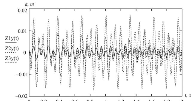
Fig. 4. Impact of the debalances masses on the magnitude of oscillation amplitude of the separator drum at  $Z1 - M_{D1} = M_{D2} = 1$  kg,  $Z2 - M_{D1} = M_{D2} = 2,5$  kg,  $Z3 - M_{D1} = M_{D2} = 4$  kg
