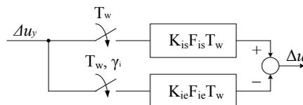
Fig. 5. Pulse model of the voltage converter for an active filter-stabilizer with a two-way pulse width modulation
