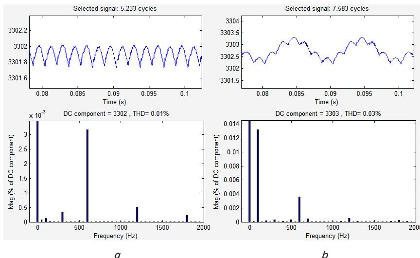
Fig. 6. Voltage pulsations and spectral composition diagrams at the output of the converter unit with AFS at symmetry (a) and asymmetry (b) of three-phase feeding voltage
