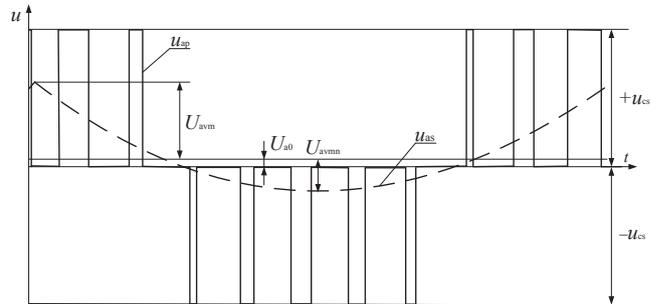
Fig. 2. Diagram of the AFS output voltage
