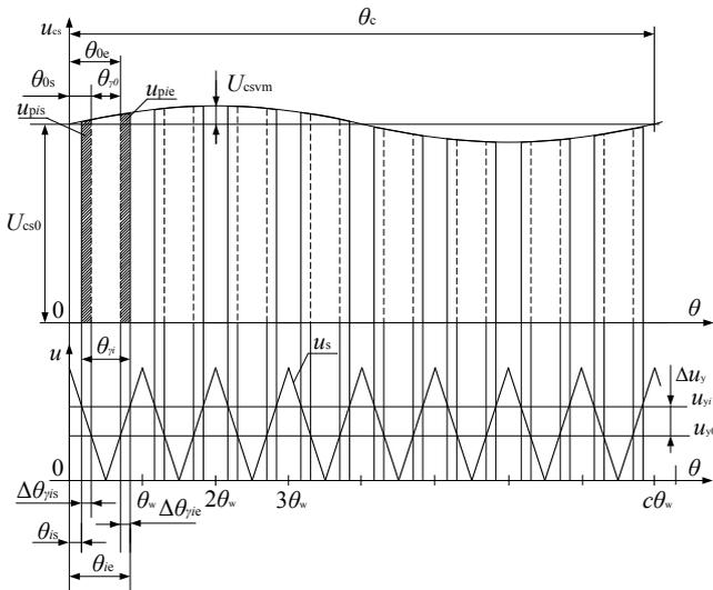
Fig. 4. Voltage diagrams in the AFS converter with a two-way PWM in a dynamic mode
