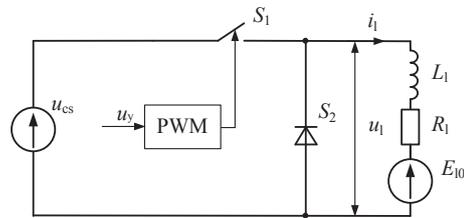
Fig. 3. Generalized equivalent circuit of the voltage converter of the active filter-stabilizer with pulse-width modulation
