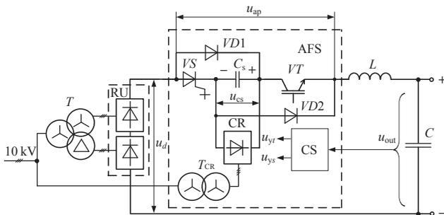
Fig. 1. Circuit of the active filter-stabilizer as a part of the traction substation converter unit
