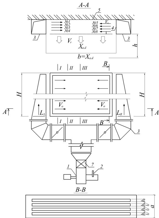
Fig. 6. Schematic of experimental plant for studying the flow, formed by interaction of counter non-coaxial flat jets, where 1 – ventilation unit; 2 – shutter; 3 – airduct of dimensions  $a \times b = 350 \times 350 \text{ mm}$ ; 4 – inflowing nozzles of width  $b_0 = 20 \text{ mm}$ ; 5 – base; 6 – constructive part of air distributor; 7 – air heater;  $h$  – distance to the characteristic plane of velocity fields
