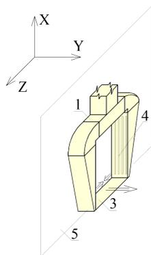
Fig. 2. Air distributor with interaction of counter non-coaxial flat jets: 1 – airduct; 2 – structural part of air distributor; 3 – structural part of air distributor; 4 – inflowing slots  $b_0=20$  mm; 5 – base
