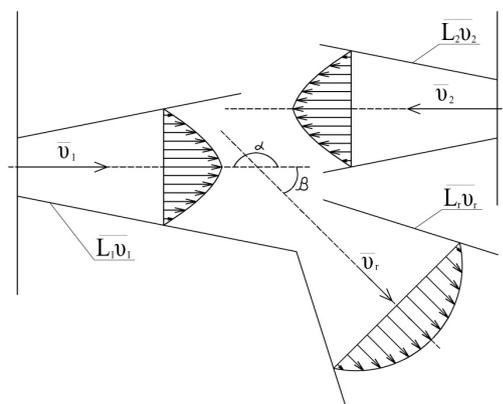
Fig. 5. Schematic of collision of counter non-coaxial jets
