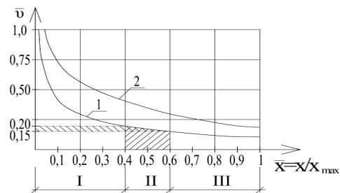
Fig. 11. Determining the jets range: 1 – for flat jets; 2 – for round jets
