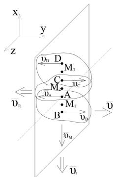
Fig. 4. Velocity vector  $\vec{v}_p$  (progressive motion) of the resulting air flow as a result of interaction of counter non-coaxial flat jets (couple of rotation) with velocities  $\vec{v}_R$  and  $\vec{v}_L$ .
