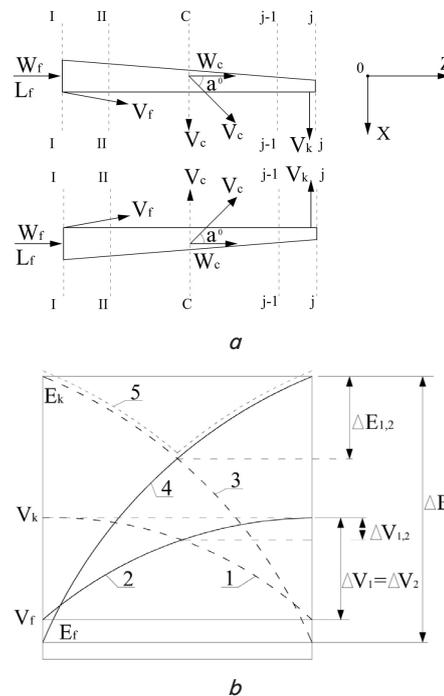
Fig. 3. Change in velocity and specific kinetic energy lengthwise the slots at the outflow of interacting counter jets; b – change in specific kinetic energy
