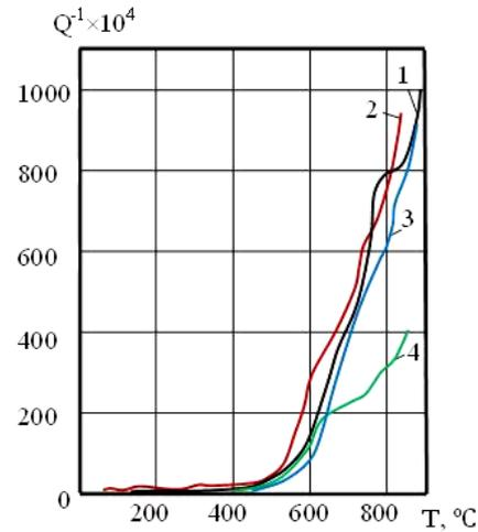
Fig. 1. Temperature dependence of internal friction in the samples of steel Cr18Ni9Ti: 1 and 3 – uncoated; 2 and 4 – plasma-coated (the coating is based on NiA1–SiO<sub>2</sub>·Al<sub>2</sub>O<sub>3</sub>); samples 1 and 2 are in the deformed state; samples 3 and 4 are preannealed before sputtering for 2 h at  $T=1100\text{ }^\circ\text{C}$
