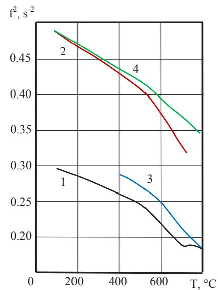
Fig. 4. Temperature dependence of the quadratic vibration frequency of the samples of steel Cr18Ni10Ti: 1, 3 – uncoated; 2, 4 – coated; 1, 2 – deformed; 3, 4 – preannealed
