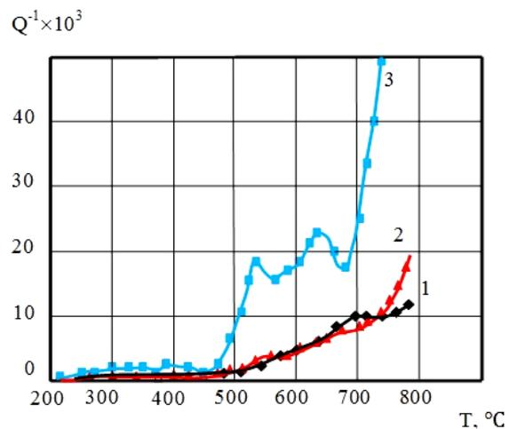
Fig. 5. Temperature dependence of the internal friction in the “steel-coating” system: 1 – the uncoated base of Cr18Ni10Ti; 2 – the base of Cr18Ni10Ti with the plasma coating ( $\text{NiAl-SiO}_2\text{-Al}_2\text{O}_3$ ); 3 – the absorption of energy in the coating
