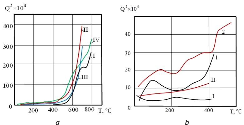
Fig. 2. Temperature dependence of IF in the capillary samples of steel 12Cr18Ni10Ti: a – I, III – uncoated; II, IV – plasma-coated (the coating is based on NiA1–SiO<sub>2</sub> Al<sub>2</sub>O<sub>3</sub>); curves I and II – deformed; III and IV – preannealed for 2 hours at  $T=1100\text{ }^\circ\text{C}$  before sputtering; b – the findings correspond to Fig. 1, 2, and on a large scale – to the temperature range of  $T=20\text{--}400\text{ }^\circ\text{C}$
