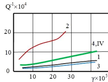
Fig. 3. Amplitude dependence of the internal friction in the samples of steel Cr18Ni10Ti: 1, 3 – uncoated; 2, 4 – coated; 1, 2 – deformed; 3, 4 – preannealed; IV – the tubular coated preannealed sample of steel 12Cr18Ni10Ti
